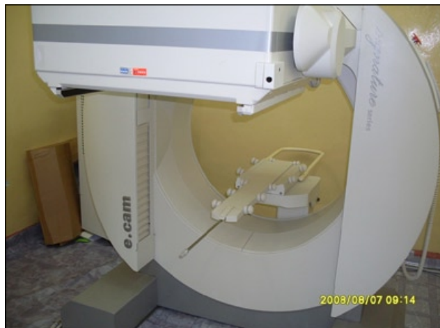
Figure 1. Set up for the Daily Flood Uniformity Test
