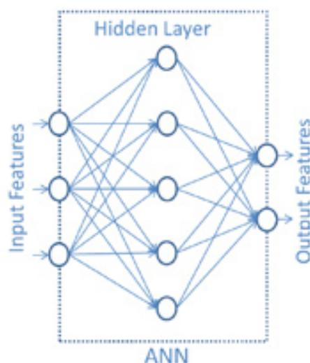
**Figure 1.** Block diagram of an ANN. The circles (neurons) represent the computation units, the connection lines represent the inter neurons connections (synapses).
