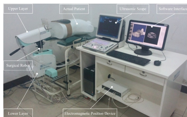
Figure 1. The general layout of the robotic prostate brachytherapy system.
