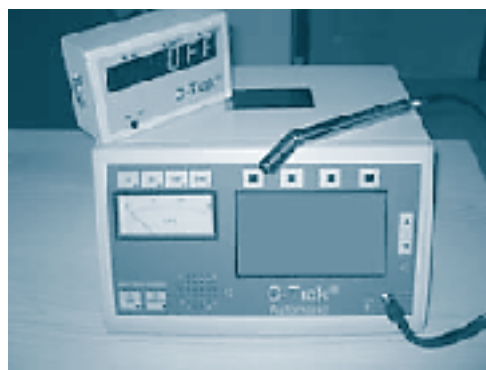
Figure 3. The gamma probe device used in GPCT.
